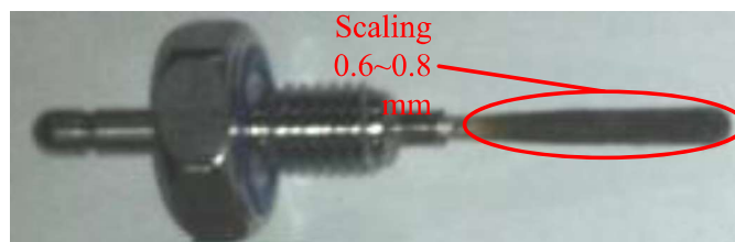
Figure 10. Deposit on grading electrodes at anode side of valve assembly of rectifier station
