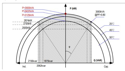
Qmax: +2156Kvar, when the power factor is +0.8, at 25°C;Qmin: -2156Kvar, when the power factor is -0.8, at 25°C;
