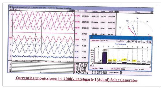
As per CEA technical Standards for connectivity to the Grid-2007 as amended, measurement of harmonic content, DC injection and flicker shall be done at least once in a year in presence of the parties concerned. However, no RE Generator has provided any such measurement report to CTU. Standard methodology may be taken into consideration for the measurement.
