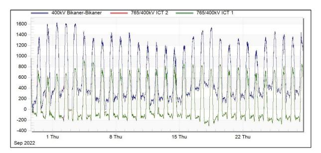
As can be seen from the plots above that the combined loading of 765/400kV Bikaner(PG) ICTs and 400kV Bikaner(PG)-Bikaner(RS) line is crossing 3000MW during high solar generation hours.
