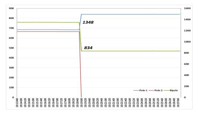
It seems from SCADA data, case-1 operated (bipole reduction by more than 750MW). However, in actual case-2 would have been operated as reduction of only ~515MW occurred as per SCADA data.
