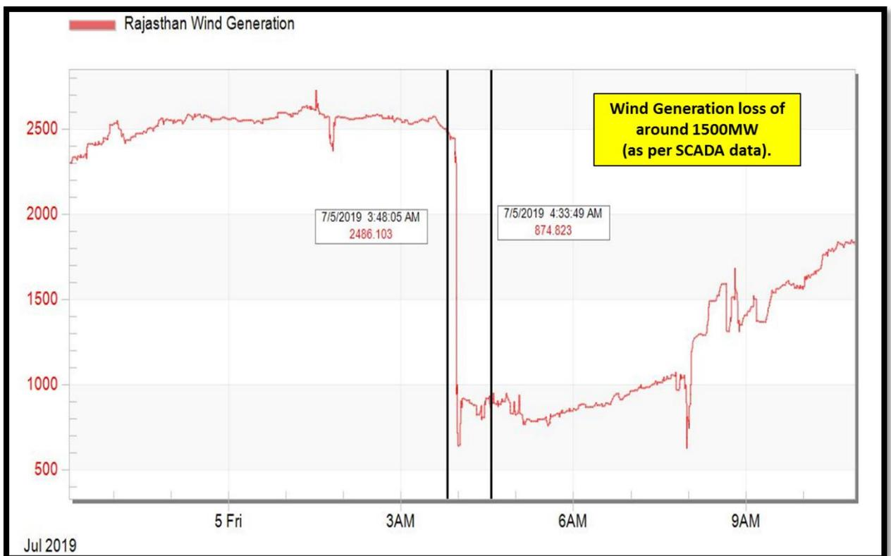
It is suspected that cause of large renewable generation tripping is due to unavailability of FRT capabilities in various wind generating stations. These large scale trippings are serious threat for security of the entire grid and also occurred in the past.
