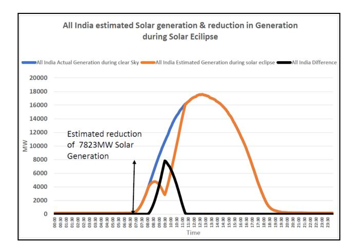
It is estimated that Northern Region PV generation would decrease by approximately 1000MW within 1.00 hour from start of eclipse and would increase by almost 2100 MW within 1:45 hrs after the maximum impact of the eclipse.
