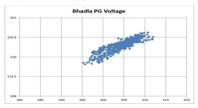
During the PSSE study, a decrement of one tap in the 400/220 kV ICTs results in an increase of 1.9 kV at the 400 kV Bhadla-PG (no change is observed in 220kV voltage), along with an approximate increase of 245 MVAr in reactive power injection. Therefore, the option of changing taps to decrease the voltage on the 400 kV side may be considered.
