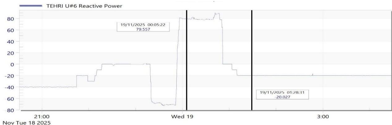
Tehri HPP tested for synchronous condenser mode of operation on 20.11.2025:
