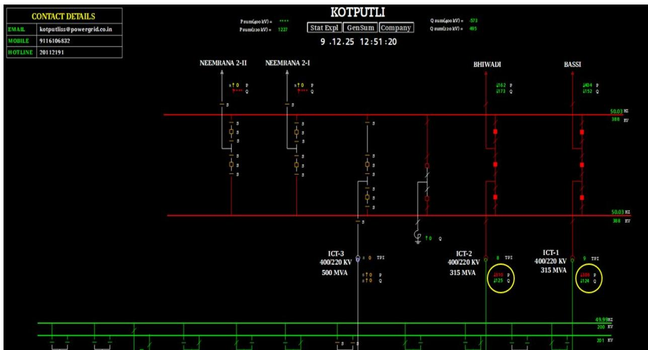
List of a few 400/220 kV ICTs in Rajasthan with loading beyond N-1 limits (Loading observed
