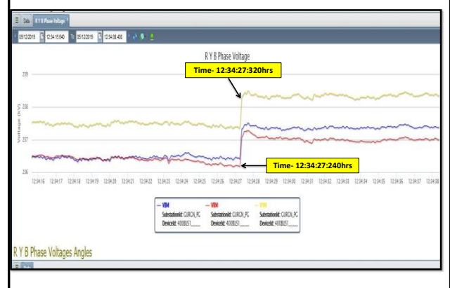
PMU Plot of phase voltage magnitude at Kota(PG) 12:34hrs/05-Dec-19
