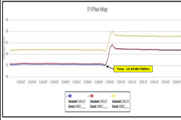
PMU Plot of phase voltage magnitude at Kota(PG) 12:29hrs/05-Dec-19
