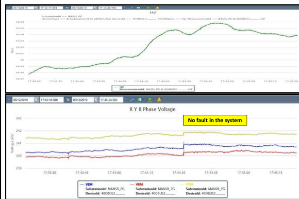
PMU Plot of phase freq & phase voltage magnitude 17:44hrs/06-Dec-19
