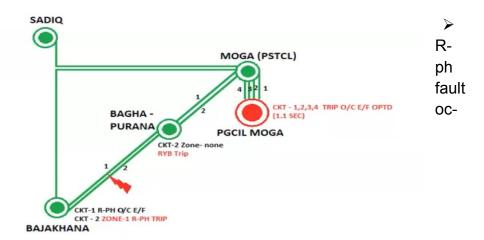
curred on 220kV Baghapurana-Bajakhana ckt. Line tripped from Bajakhana end in Z-1 however, line didn't trip from Baghapurana end as distance protection was blocked due to damage of VT control cable.
