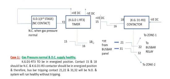
Proposal to remove K.G.D 1 RT3 timer has been sent to relay engineer to avoid operation of bus bar protection during DC supply changeover. Issue related to unwanted operation of bus bar protection will be resolved after this.
